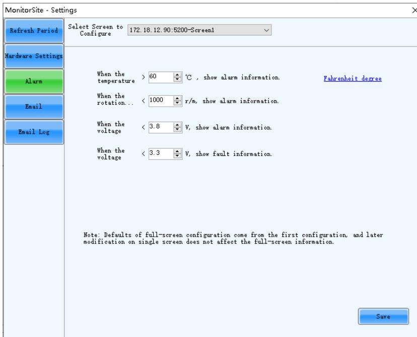
Set the alarm thresholds for temperature, fan rotating speed and voltage. When the threshold value is exceeded, faults or alarms will be displayed. After the configuration is done, click **Save** to save the settings.
