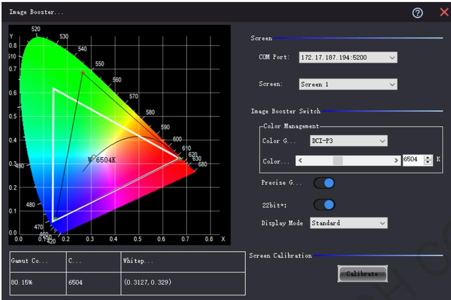
If the connected receiving card supports the 18bit+ function, the **22bit+** displayed on the user interface will become **18bit+**. The **22bit+** user interface is used as an example in all the following operations.
