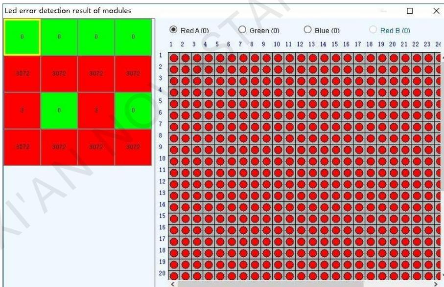
Step 7 Select a red module, and select **Red A**, **Green**, **Blue** or **Red B** (virtual red) on the right to view the faulty LED lights which are shown in black.
