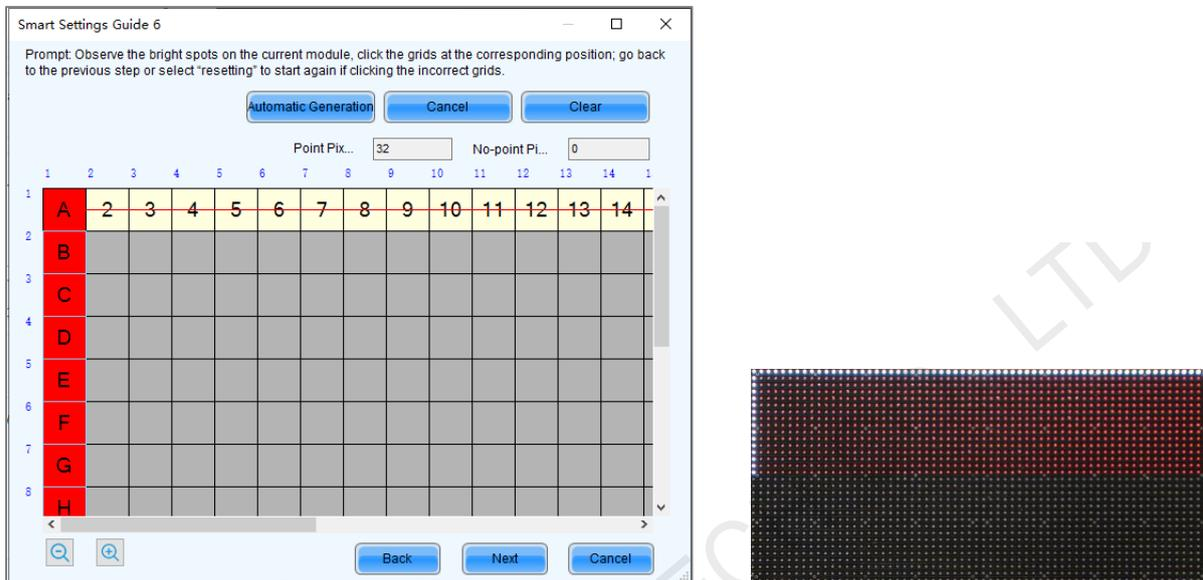
Step 13 View the flashing pixel in the first column on the module and click the corresponding cell in the grid to draw the pixel position (You can also use the keyboard arrow key to quickly draw the position), and click **OK** after the drawing is done.
