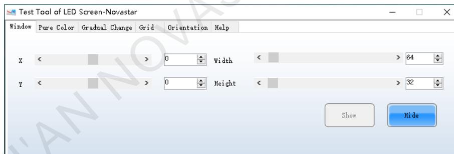
Step 4 Select the **Pure Color**, **Gradual Change**, **Grid** or **Orientation** tab to set the test pattern style.
