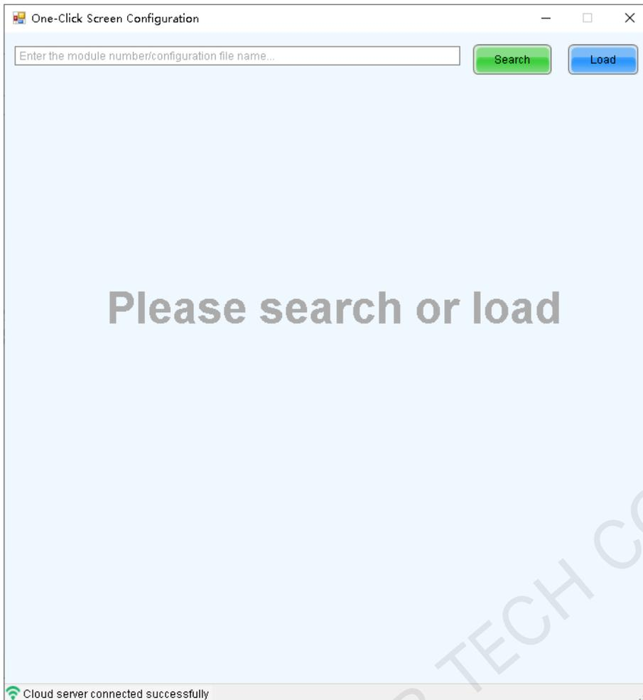
In the bottom-left corner of the page, the status of connection between NovaLCT and cloud platform is displayed.
