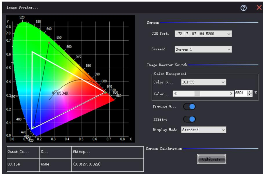
Step 4 Set the color gamut, color temperature and 18bit+ switch, and view the effect on the screen.
