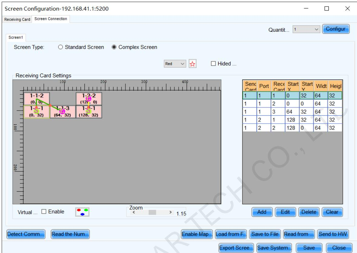
Step 8 Click **Send to HW** to send the configuration information to the hardware. If necessary, click **Save to File** to save the configuration information as a file.
