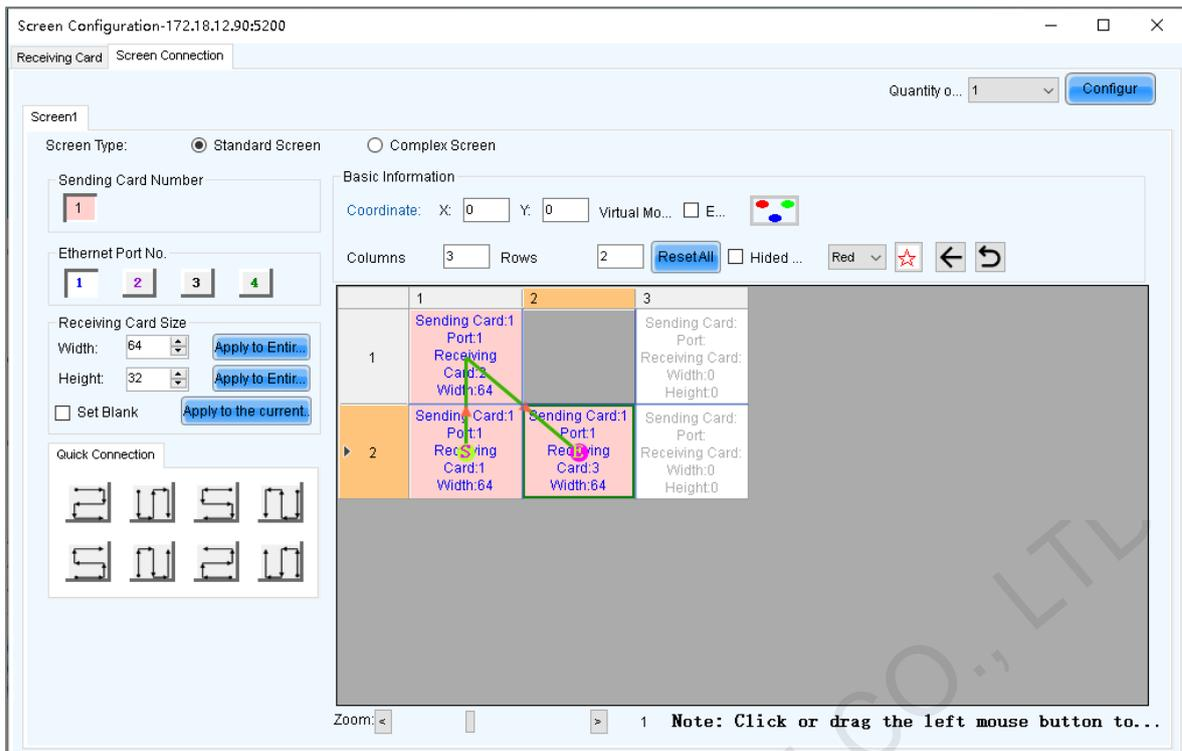
Step 7 Repeat [Step 4](#) to [Step 6](#) to set the receiving cards loaded by the other output ports.
