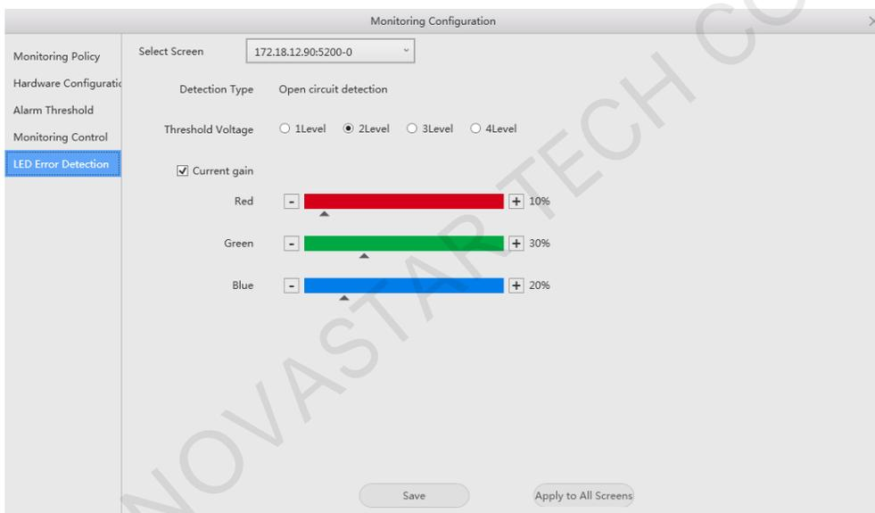
Set the LED error detection parameters. After the settings are done, click **Save** or **Apply to All Screens**.
