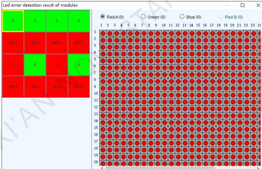
Figure 9-7 Result of the Led error detection for all the modules
