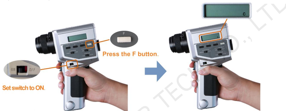
Figure 12-7 Setting CS-100A colorimeter
